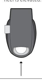
Apply one or two optional wedges to outside/inside of boot for extra stabilization.
